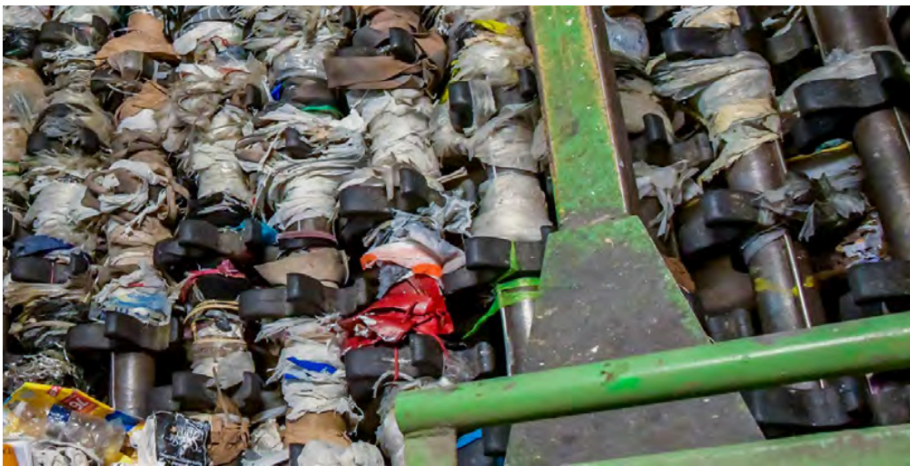
Employees removing tangled plastic bags from recycling equipment
